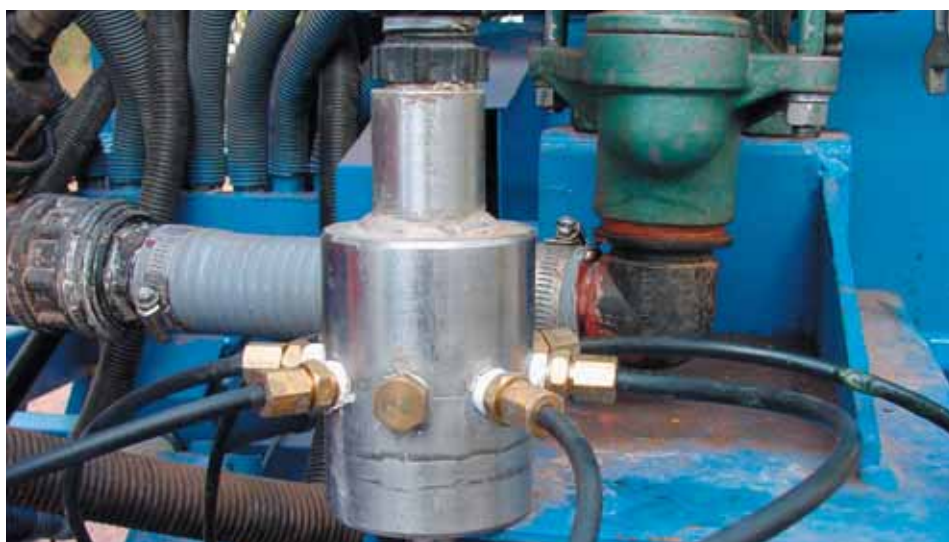
Figure 5. Anhydrous ammonia distributor used on an experimental seeder for fluid fertiliser distribution.
