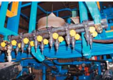
Figure 3. Distribution manifold showing non-drip nozzle fittings housing orifice plates to control pressure and flow.
